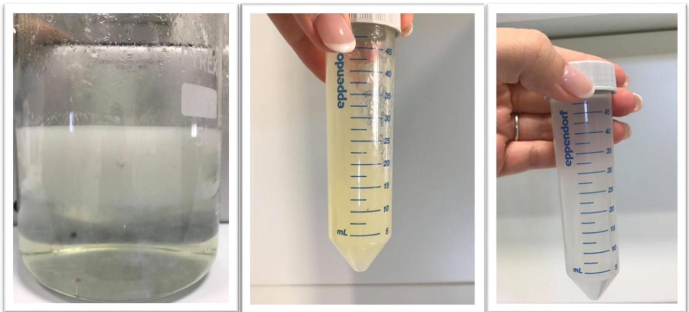
Figure 3 Left: Salt precipitation of acid solubilised collagen from bone, Middle: Acid solubilised collagen dialysate from muscle, Right: Pepsin solubilised collagen dialysate from bone.
